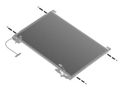
Where used: 4 screws that secure the display hinges to the display panel
